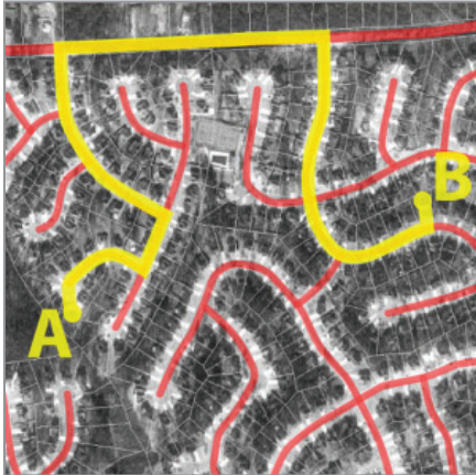
In a dendritic system, the distance from A to B is one mile, achievable only along one route
