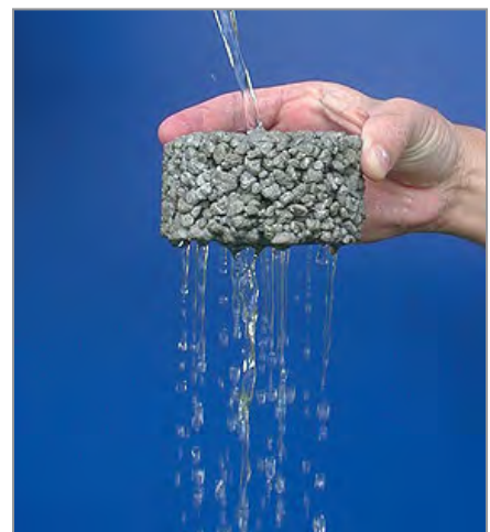
Pervious paving allows water to pass through it and infiltrate into the ground
