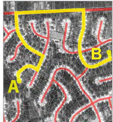
In a dendritic system, the distance from A to B is one mile and achievable along one route
