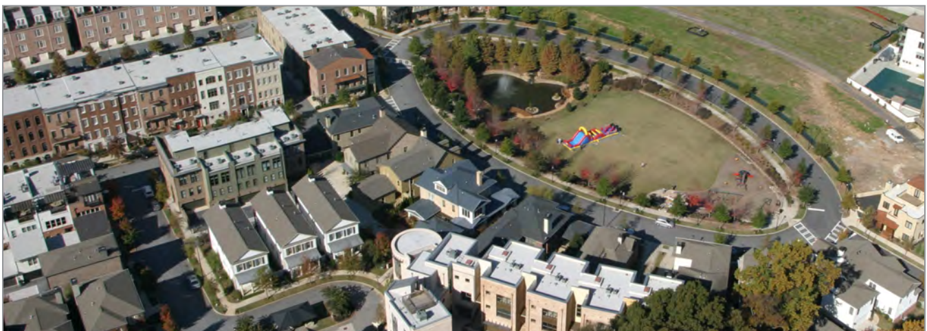
At the Glenwood Park in Atlanta a shared stormwater facility (above right) serves multiple building sites and doubles as a park space. During periods of heavy rain the green lawn above fills with water. The rest of the time it is a highly-used public park. A similar model should be explored on the GM site.
