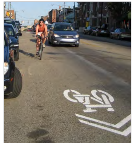
Sharrow markings are used where there is not room for bike lanes
