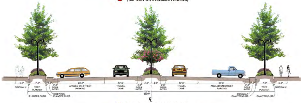
9 PROPOSED STREET SECTION 9 (105' ROW WITH ANGLED PARKING AND LANDSCAPE MEDIAN)
