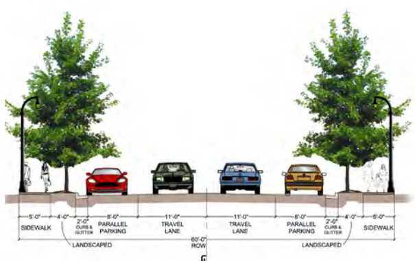
5 PROPOSED STREET SECTION 5 (60' ROW WITH PARALLEL PARKING)
